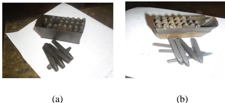
Fig. 4a & 4b: Letter Punches used by the Goldsmiths
