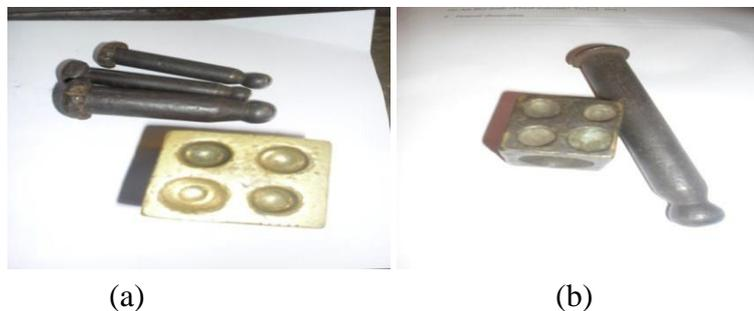
Fig. 3a & 3b: Samples of doming blocks and metal Punches used by the goldsmiths
